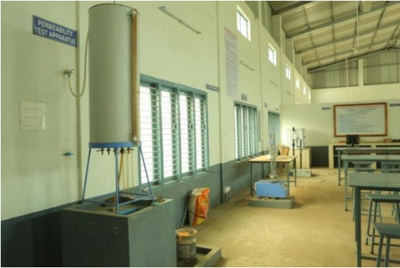
Overhead Tank for conducting Permeability of course grained soil
