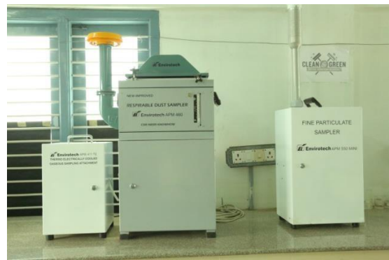
RESPIRABLE DUST SAMPLER APM 460
